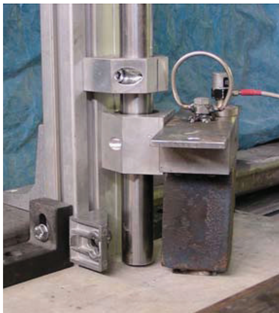
Fig. 8 View of the “drop hammer” pilot-scale measuring device.
